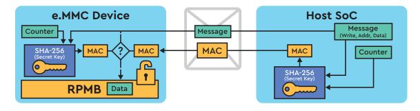
Figure 2: RPMB Write Sequence Block Diagram
