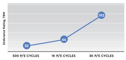
**Figure 2.** Endurance Rating vs. P/E Cycles
