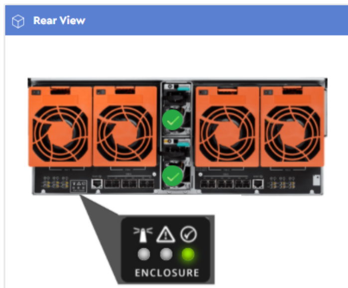
Figure 59: Identification LEDs Disabled
