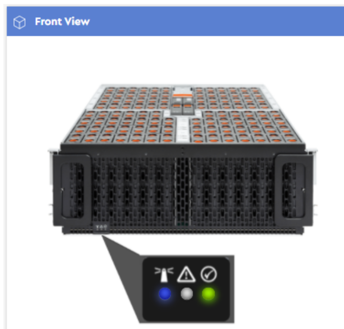
Figure 52: Identification LEDs Enabled
