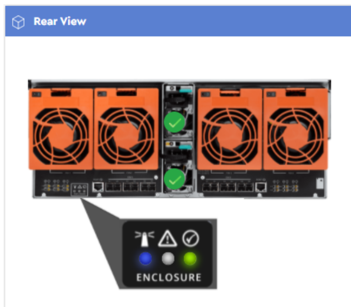
Figure 58: Identification LEDs Enabled
